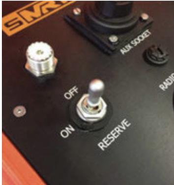
1. Lift to move the MASTER ON / OFF / RESERVE switch from [OFF] to [ON].
