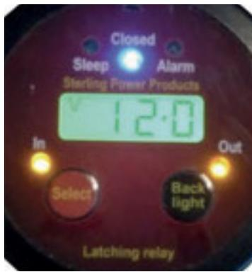
If the AGM **BATTERY** voltage drops to 10.9 volts during normal operation, the unit will shut down to prevent deep discharge of the battery. During a recovery operation this can be overridden by moving the **MASTER ON / OFF / RESERVE** switch to the **[RESERVE]** position. This will allow the unit to continue operation.
