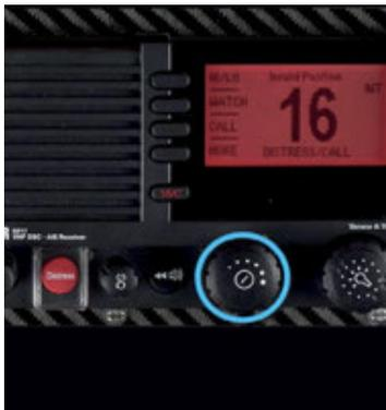
2. Press the VOLUME WHEEL KNOB to turn the radio [ON].
