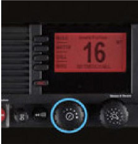
1. Press and hold the **VOLUME WHEEL KNOB** for 3 seconds to turn the radio [**OFF**].
