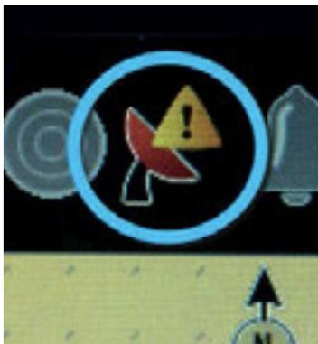
2. Initially the GPS satellite symbol will indicate no satellite lock has been acquired.
